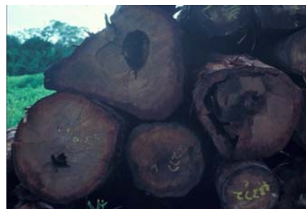
Photo: 14 - Native rain forest trees "piped" by Neotermites Photo: Dr Michael Lenz
