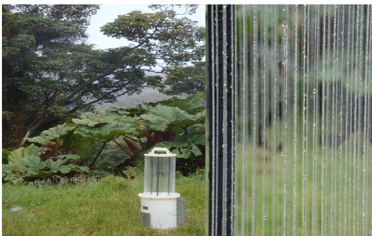
Figure 2 Photographs of the fog sampler deployed on Volcano Poas (left) and of the Teflon strings that serve to force coalescence of fog droplets.
