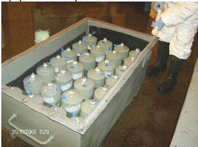
Figure 2 Shipping container with flasks of by-product mercury in preparation for transport from Yanacocha
