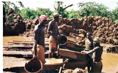
Concentration of gold ore with sluice boxes in Tanzania
